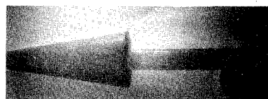
Fig. 7 Electron beam view of exhaust plume interaction with conical flowfield.
